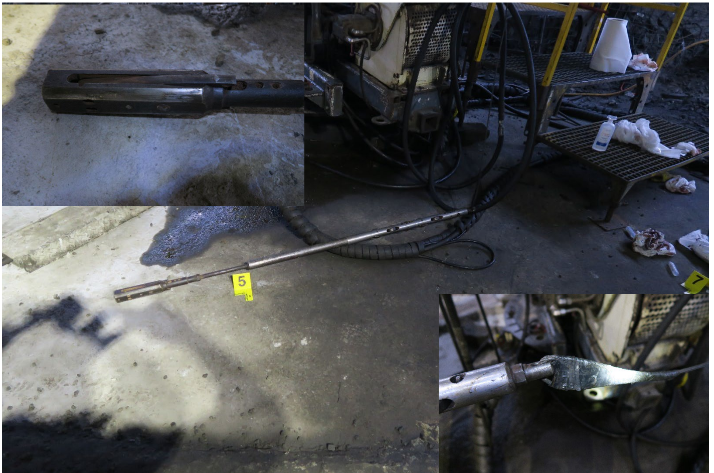
Figure 2: Photo of the overshoot with inner pictures of the locking pins and cable connection
