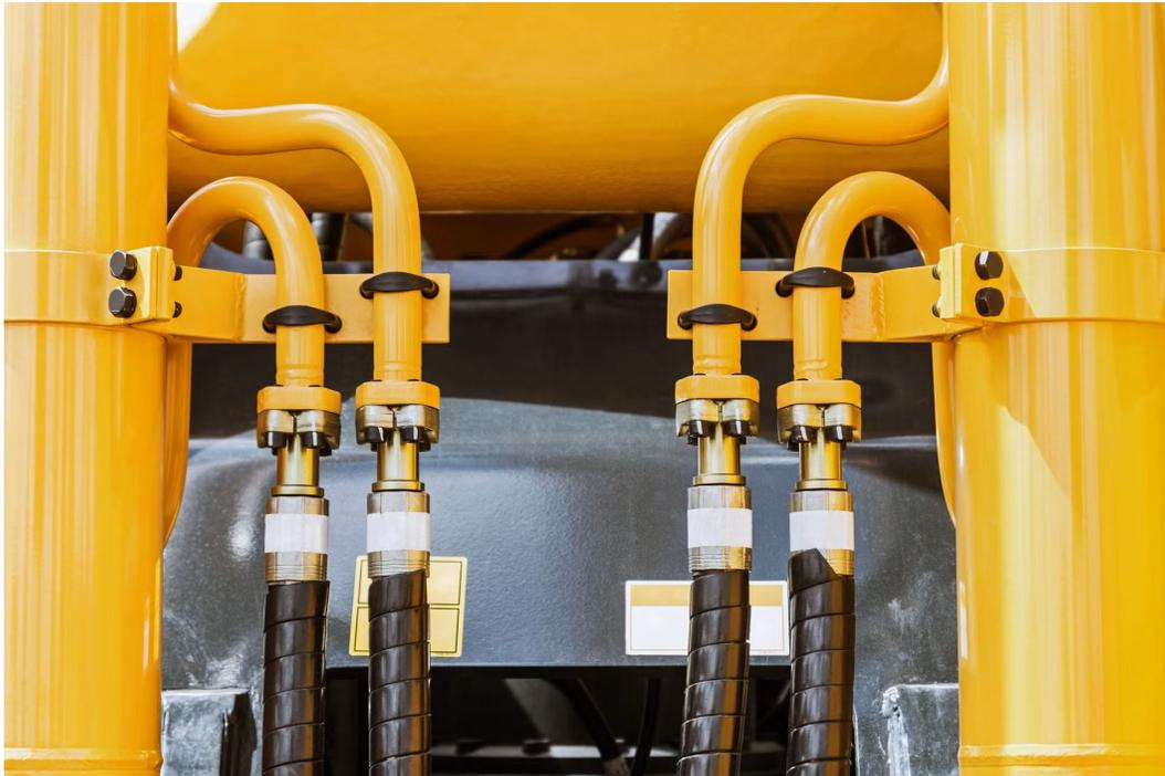
Spiral wrapping prevents rubbing wear and good clamping segregates hoses
