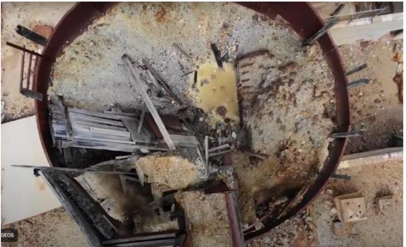
**Figure 4.6** Aerial view showing weathered ore inside of the Surge Bin, located within the Central Mine Area
