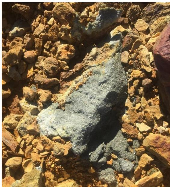
Figure 3.2 Partially oxidised sulfidic waste rock in Mill Area
