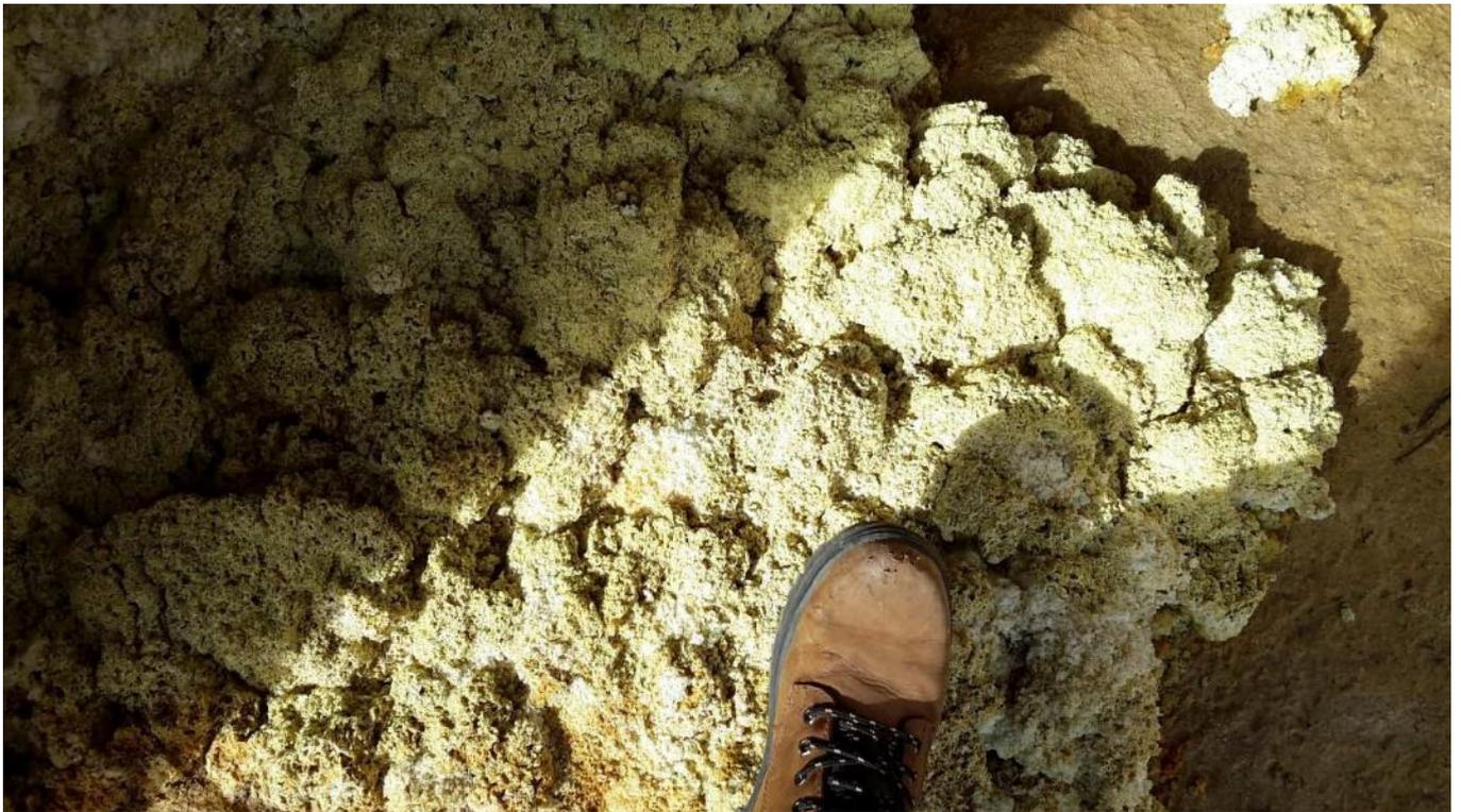
**Figure 4.5** Sulfate efflorescence outside fenced area beneath northern Concentrate Bin
