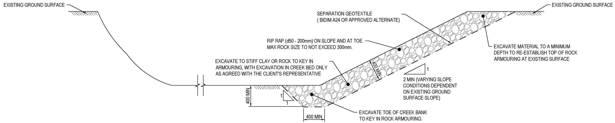
**A** TYPICAL ROCK ARMOURING - TYPE A
