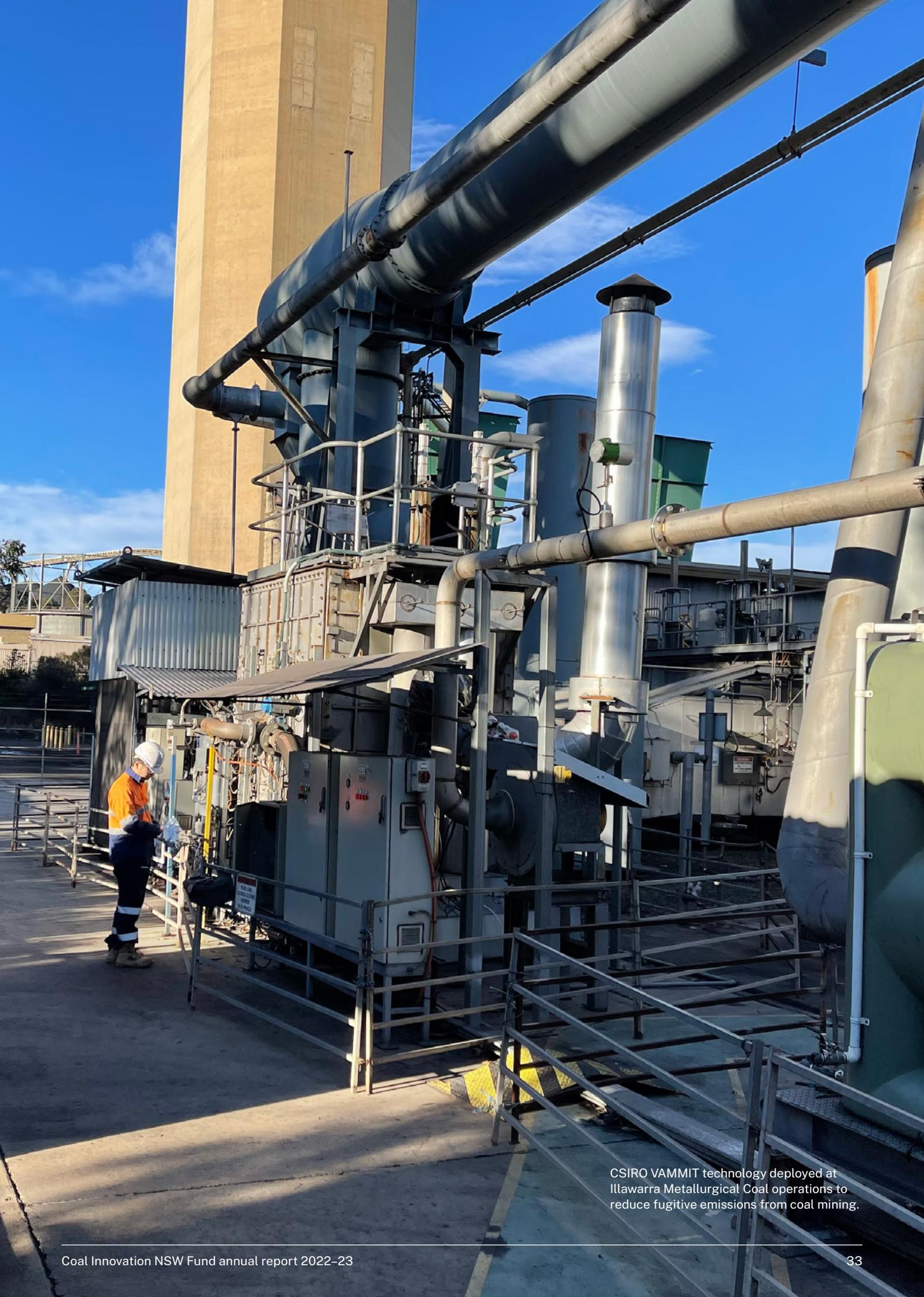
CSIRO VAMMIT technology deployed at Illawarra Metallurgical Coal operations to reduce fugitive emissions from coal mining.
