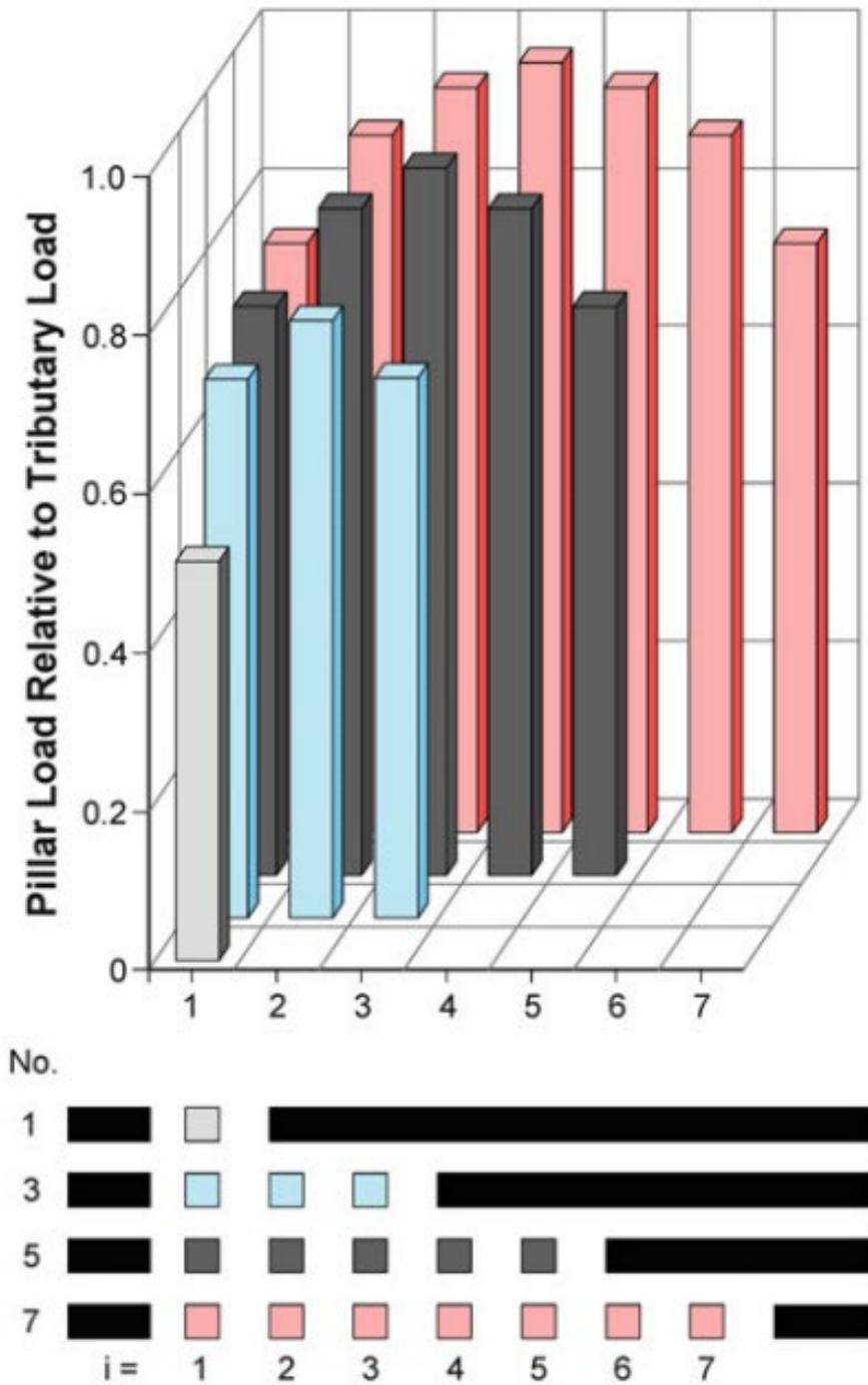
The loads acting on pillars in the centre of a panel of pillars generally approach full deadweight loading once overall pillar panel width ( $W_p$ ) exceeds 1–1.5 times depth. Larger panel spans may be required to achieve full deadweight loading when the overburden contains massive, stiff strata.
