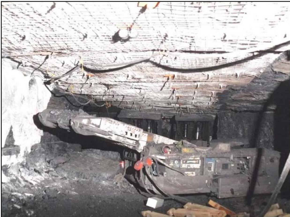
Figure 40 - Photo of incident scene from inbye of the miner showing rib slabs
