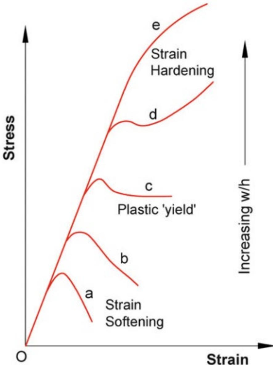
Figure 8 above shows the way that pillar width-to-height ratio influences its behaviour. After a pillar with a low width-to-height ratio exceeds its maximum resistance to deformation, it undergoes strain softening and progressively and permanently unloads with ongoing displacement. This is depicted by curve (a).
