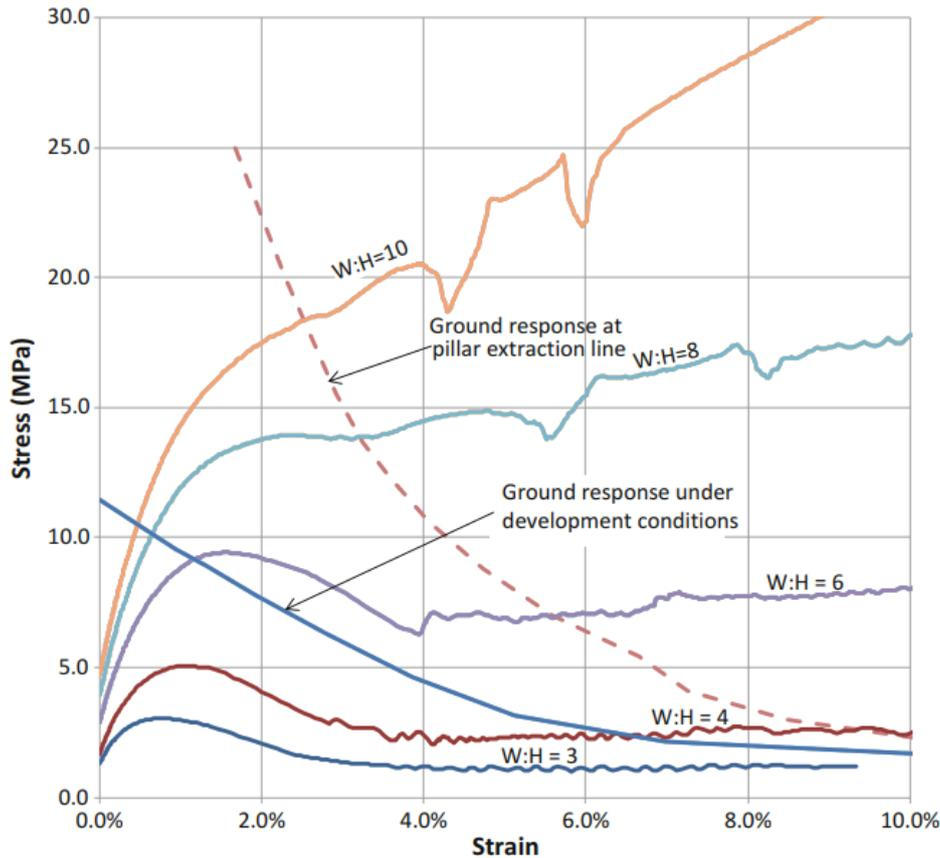
The modelling predicts that pillars with a width-to-height ratio of 8 would be in a pre-peak stress state under development conditions. Post-peak yielding occurs as the extraction line approaches and the pillars are loaded beyond their initial peak. At these relatively high stress values, the ground response is stiff, and equilibrium is reached at a vertical strain value of 3.2%.
