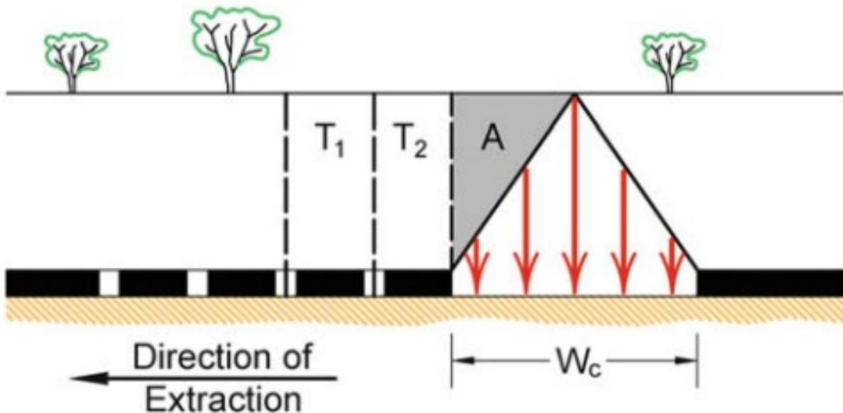
Bridging superincumbent strata can adversely affect pillar extraction operations because it increases abutment stress and the propensity for windblast and gas inrush<sup>23</sup>.
