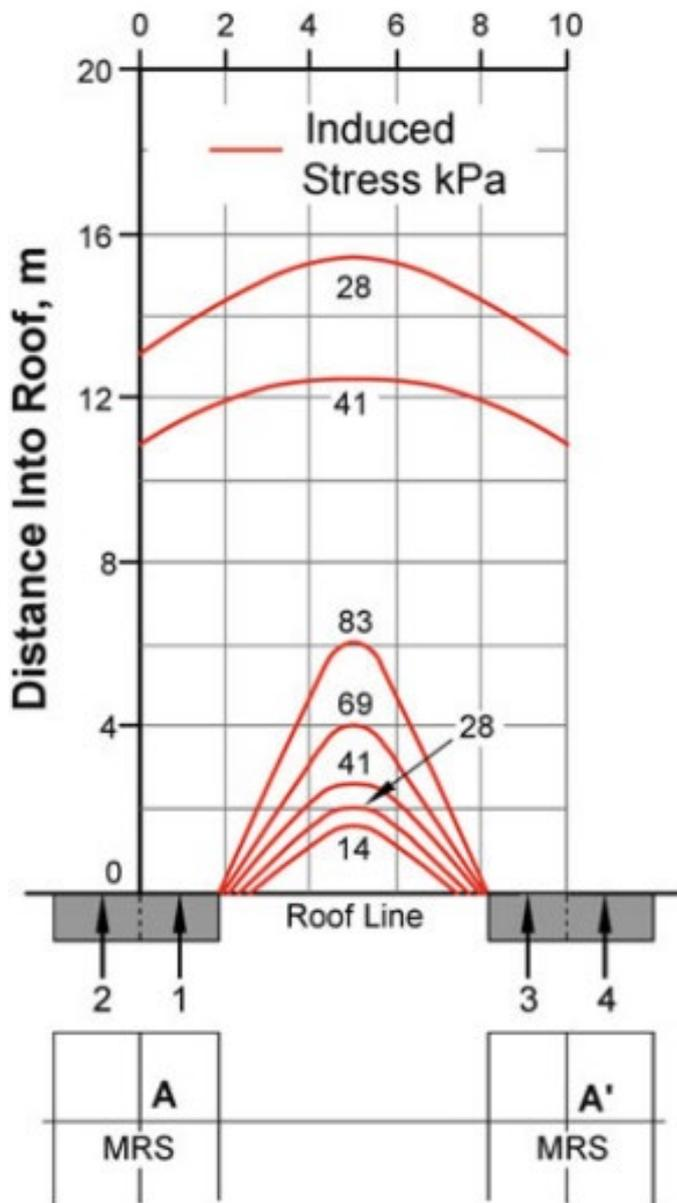
The example analysis in Figure 13 predicts that the units generate more than 40 kN (4 t) of upward force per square metre some 12 m up into roof between the midpoint of the pairs of MRS.
