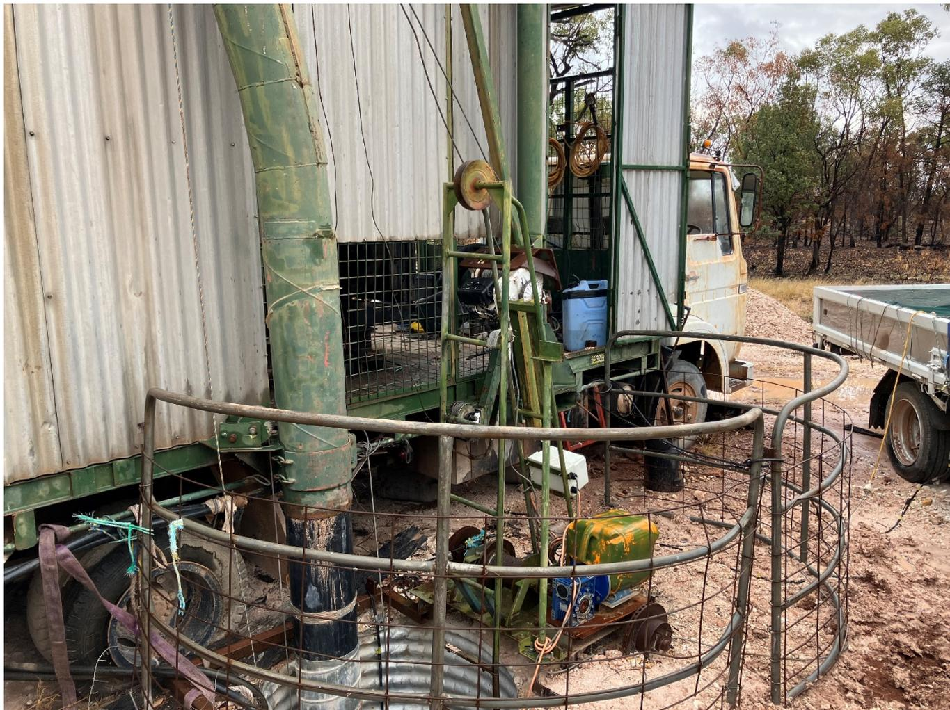
Figure 2: Cable from hoists drum was found completely unspooled
