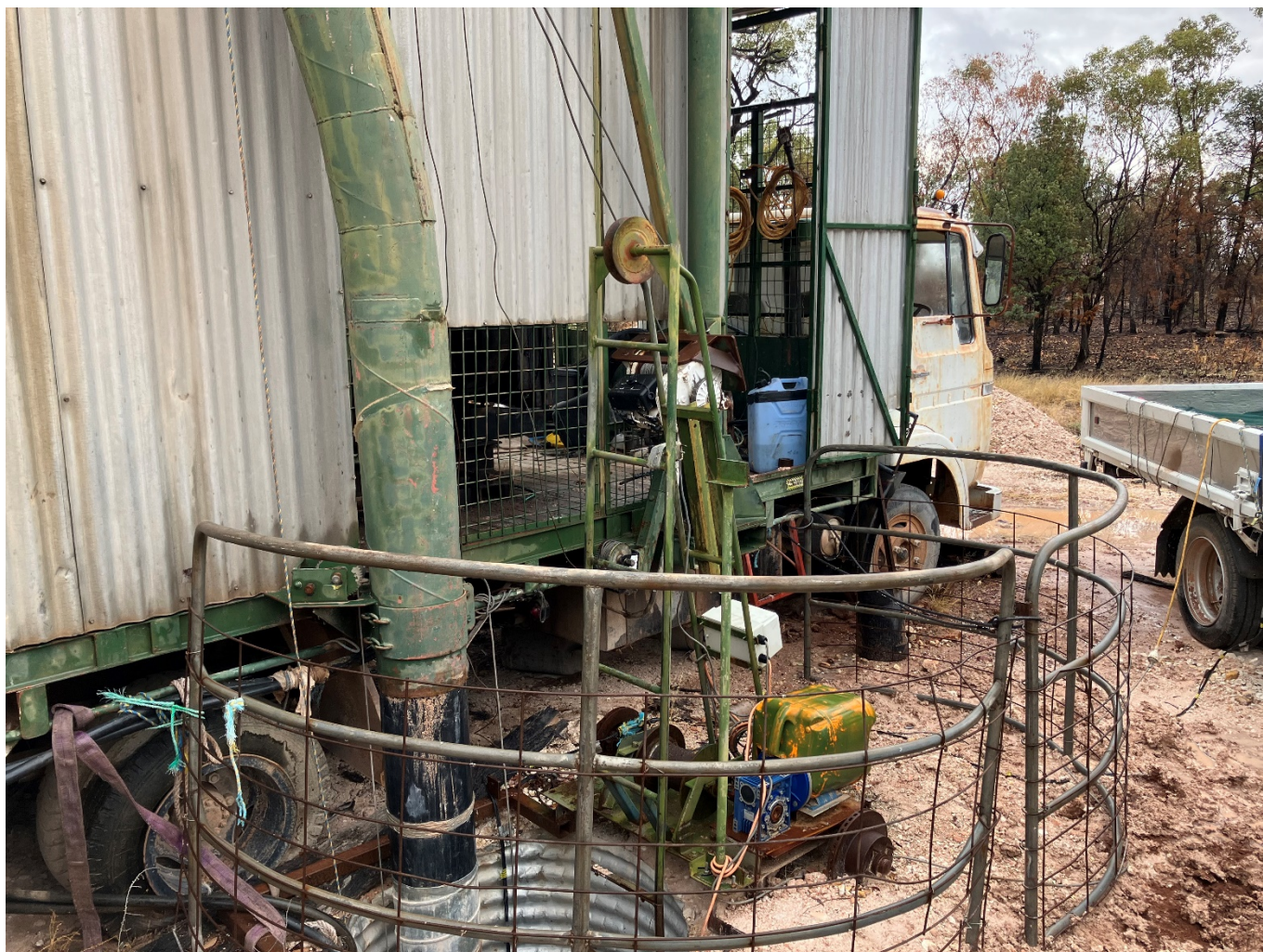
Figure 1: MC 61376 with hoist and ladder/rails to person riding hoist
