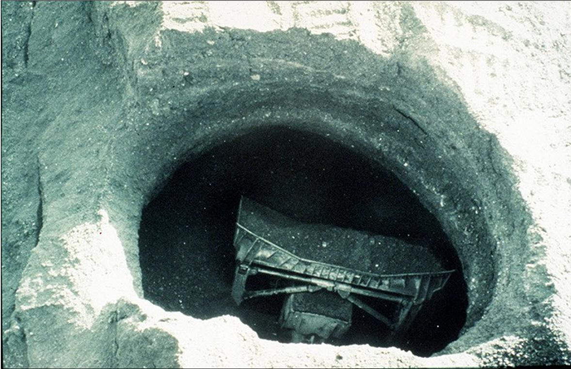
If the windows of the stockpile dozer cab are not designed to withstand the burial forces applied, material can flow into the dozer operator's cab, placing the dozer operator at risk of engulfment, suffocation, and death.
