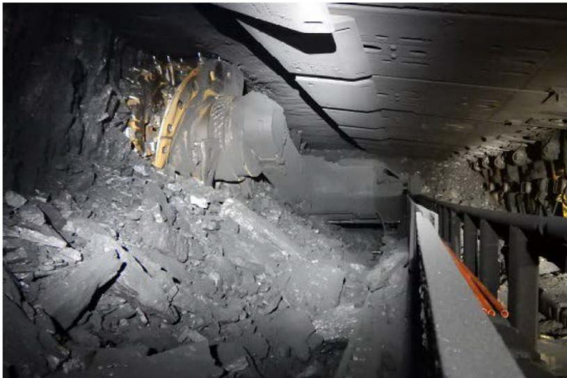
Figure 2: Tailgate view of gas outburst. Supplied by Metropolitan Colliery.
