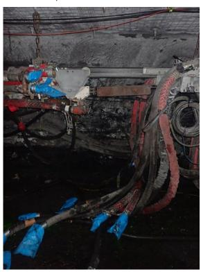
Dangerous incident IncNot0043982 Underground coal mine A worker was operating a rib bolter on a continuous miner when a hose failed. The worker was hit on the forehead and arm with hydraulic oil. The worker was assessed at hospital and cleared of injury.
