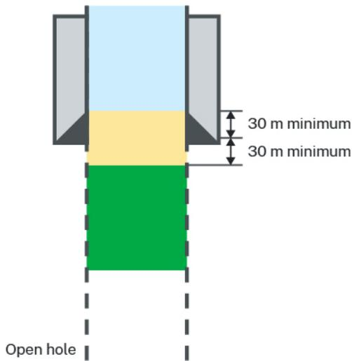
Figure 2: Casing shoe with open hole below (with lost circulation) or casing shoe with uncemented liner below
