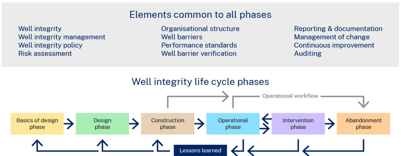
Monitoring and maintenance is required to preserve the well in a suitable condition for its useful life. Well integrity management systems and associated documents for subsurface assets aim to ensure that wells meet operational availability objectives and well integrity goals for the full lifecycle of the well.
