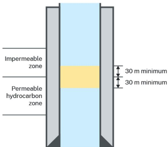
Figure 5: Casing shoe or equivalent with open hole/ uncemented liner below
