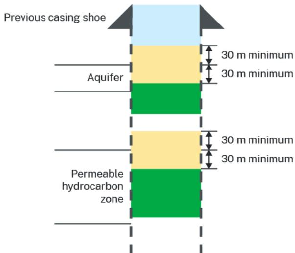
Figure 4: Cased hole section
