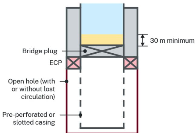
Figure 3: Cut and recovered casing/liner
