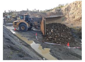
The stability of articulated vehicles is a known risk that needs to be managed at mine sites. Areas where loads are dumped should be constructed and maintained to ensure stable operations when tipping occurs. Refer to:
