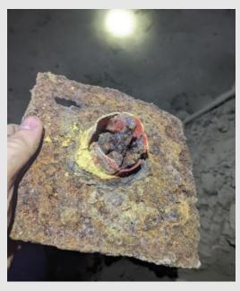
Underground mine operators should review the adequacy of support that was installed historically under different support regimes. The review should check that the age of installed support is taken into account and that the support continues to be effective.
