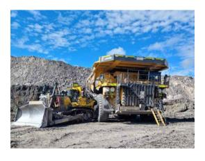
Vehicle collisions on mine sites continue to be a source of concern. As technology evolves and develops, mine operators should routinely review proximity detection and collision avoidance systems to determine if they are suitable for their operation. Workers should use all aids such as mirrors, cameras and awareness systems that are fitted when operating plant, particularly when reversing.
