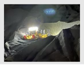
Workers must be trained to operate dozers on reclaim stockpiles. This training must include identifying and responding to alarms and managing the hazards associated with draw down valves.
