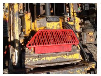
Picture shows a new guard covering pinch points
