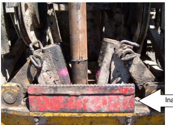
Picture showing rod clamps in open position with existing but apparently inadequate guard (worn red colour). The rod spinner is removed for clarity.
