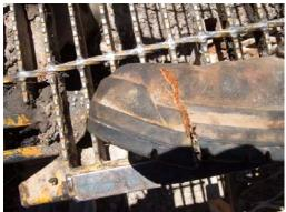
by placing his foot on the rod clamp guard to begin the removal of rods. When the rod clamp was closed the off-sider's right foot was dragged down by the closing action of the rod clamps. This resulted in a tear behind the steel cap of the boot which nearly removed his big toenail.
