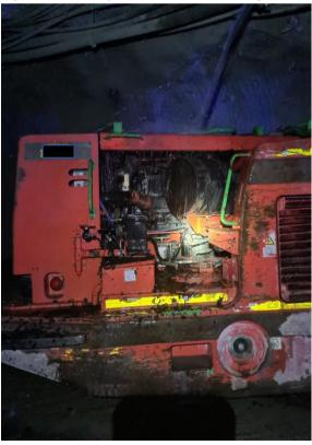
Figure 2: Loader fire location and damage
