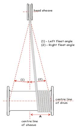
Examples of minimum rope length between the sheave had the drum with a maximum 3° fleet angle.
